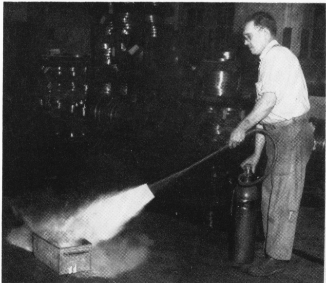
Stanley Jurzyk, of the Blanking Room, uses a hand extinguisher for a small fire.
